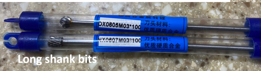
Small ball bit from drill master rotary tool Fits in locking block front leg area
