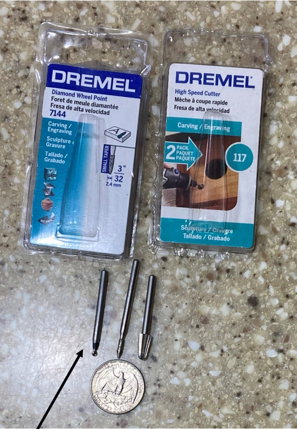
Small ball bit from drill master rotary tool Fits in locking block front leg area
